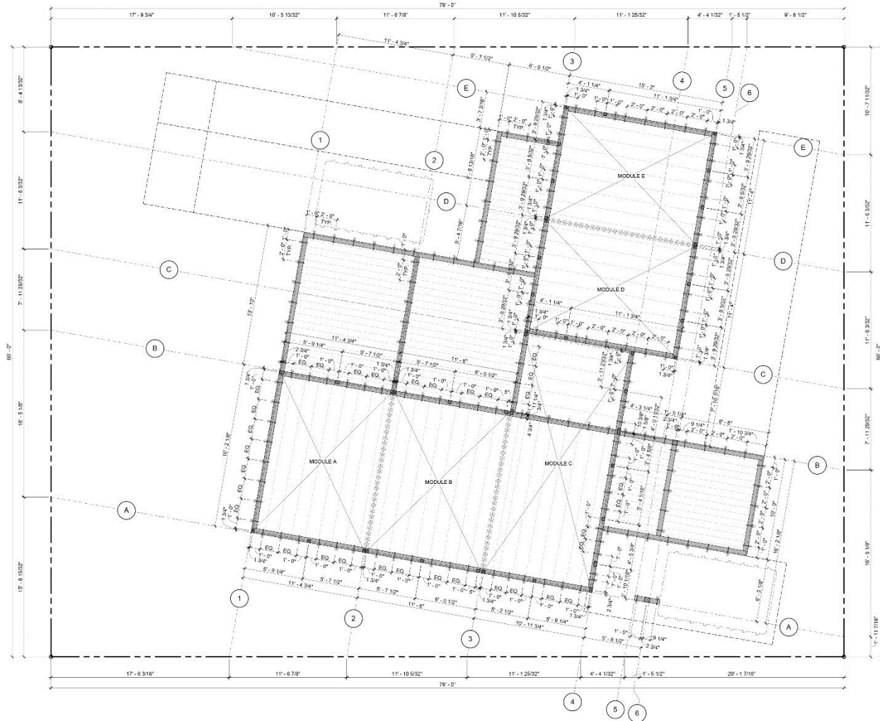
Figure 50. Temporary grade beams and foundation stakes, in plan (A1/A-105).
